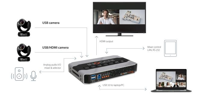
Easily switch between up to 14 video mixing configurations at the click of a button.
