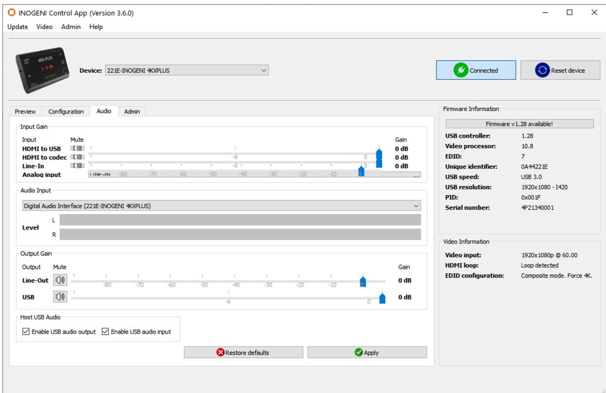
Input Gain: Control of audio gain for HDMI and Line-In.
