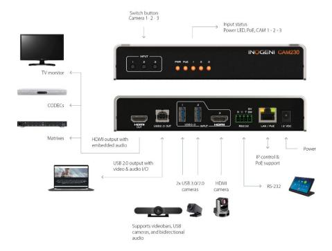
Overall, the INOGENI CAM230 is the perfect solution for meeting equity in virtual meetings. With its easy-touse camera switching capabilities, support for bidirectional audio with videobars, and support for whiteboard and document cameras, the CAM230 is a valuable tool for fostering collaboration and productivity in any virtual setting.
