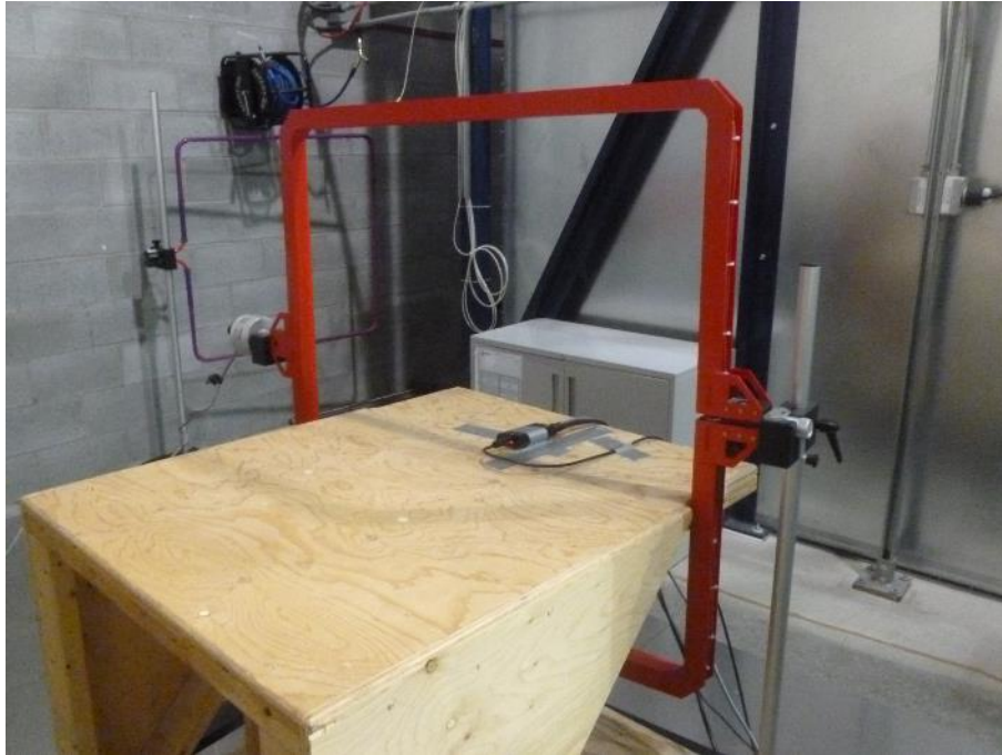
Photo 35: Magnetic Field – Test Setup – RKX-PLUS – Position #1
