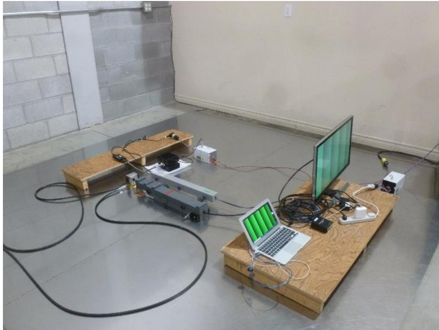
Photo 31: Conducted Disturbances – Test Setup
