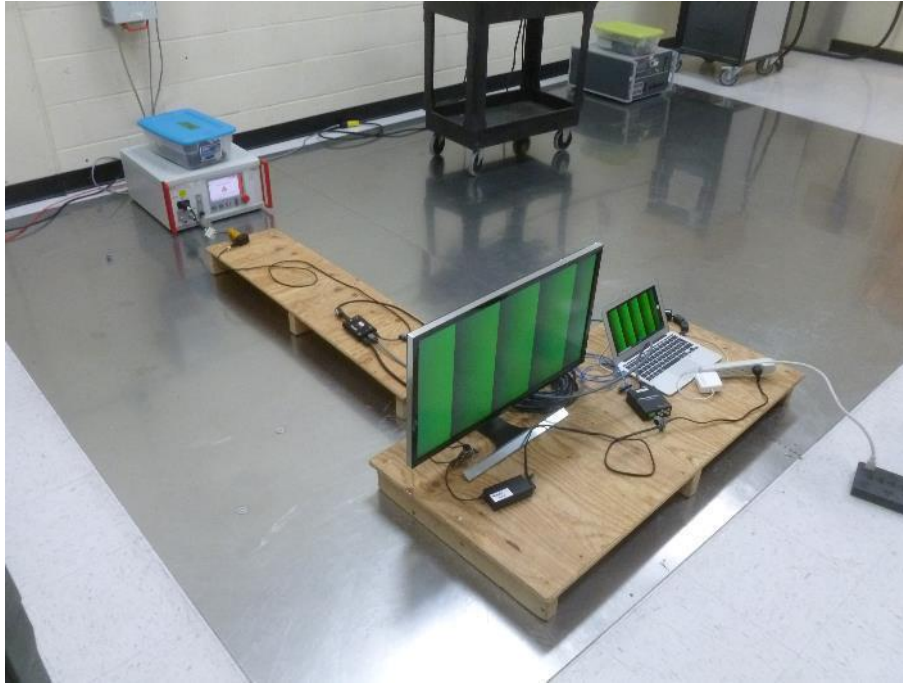
Photo 41: Voltage Variations on AC Input – Test Setup
