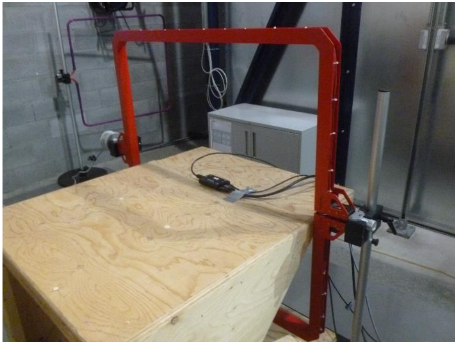
Photo 36: Magnetic Field – Test Setup – RKX-PLUS – Position #2
