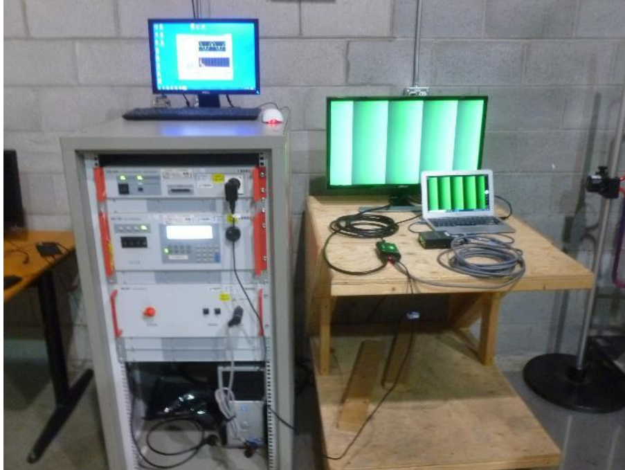
Photo 13: Harmonic Current Emissions – Test Setup
