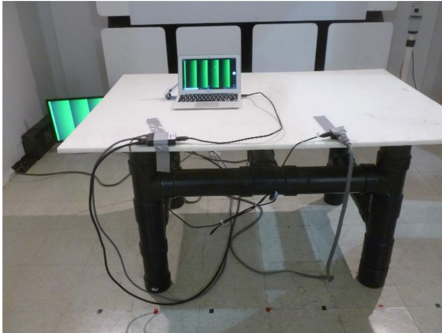
Photo 21: Radiated EM Field – Test setup – Rear
