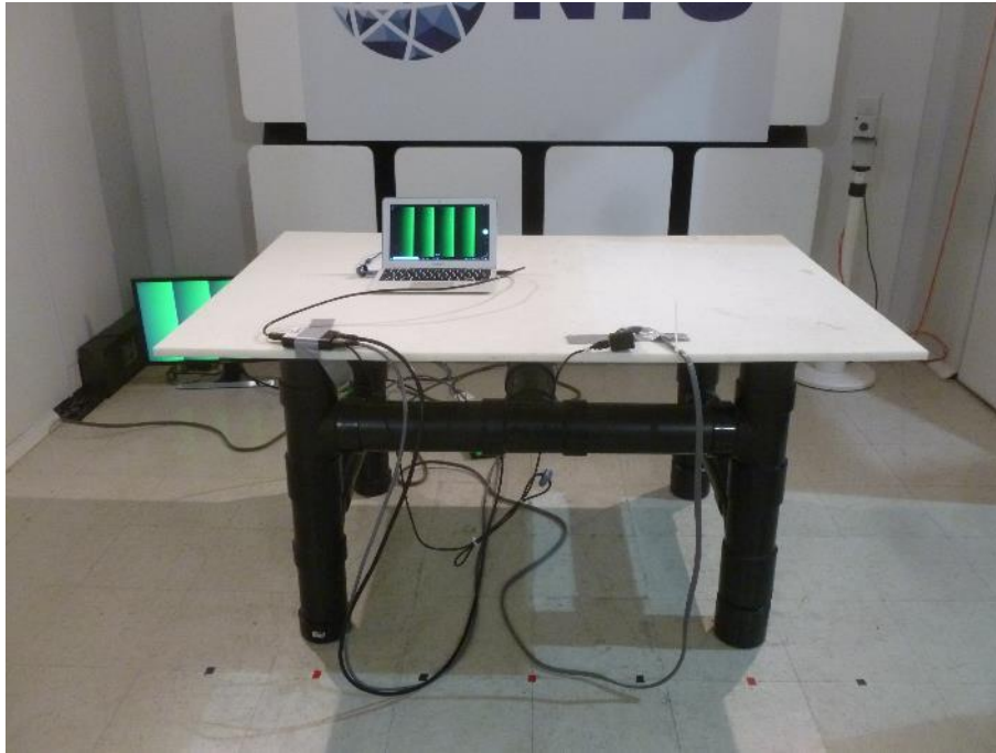
Photo 19: Radiated EM Field – Test setup – Front
