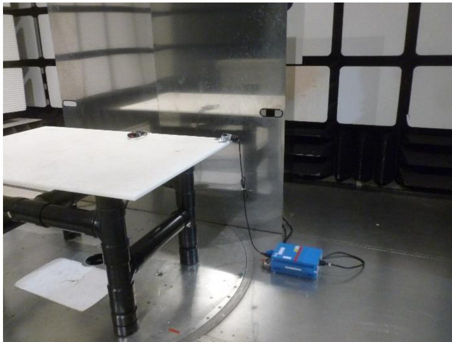
Photo 8: Conducted Emissions – Test Setup
