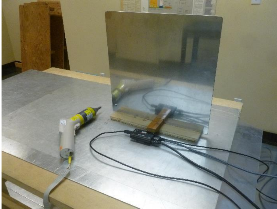
Photo 14: ESD – Test Setup – 4KX-PLUS
