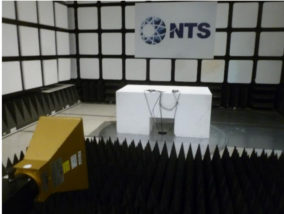
Photo 11: Radiated Emissions – Test Setup 1GHz-2GHz
