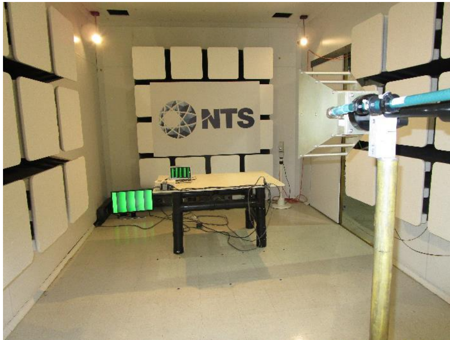
Photo 25: Radiated EM Field – Test setup – >3GHz
