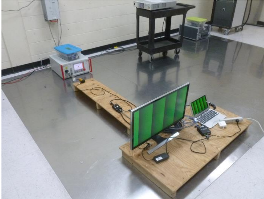
Photo 30: 1.2/50 \mu s Surge – Test Setup – Power Ports
