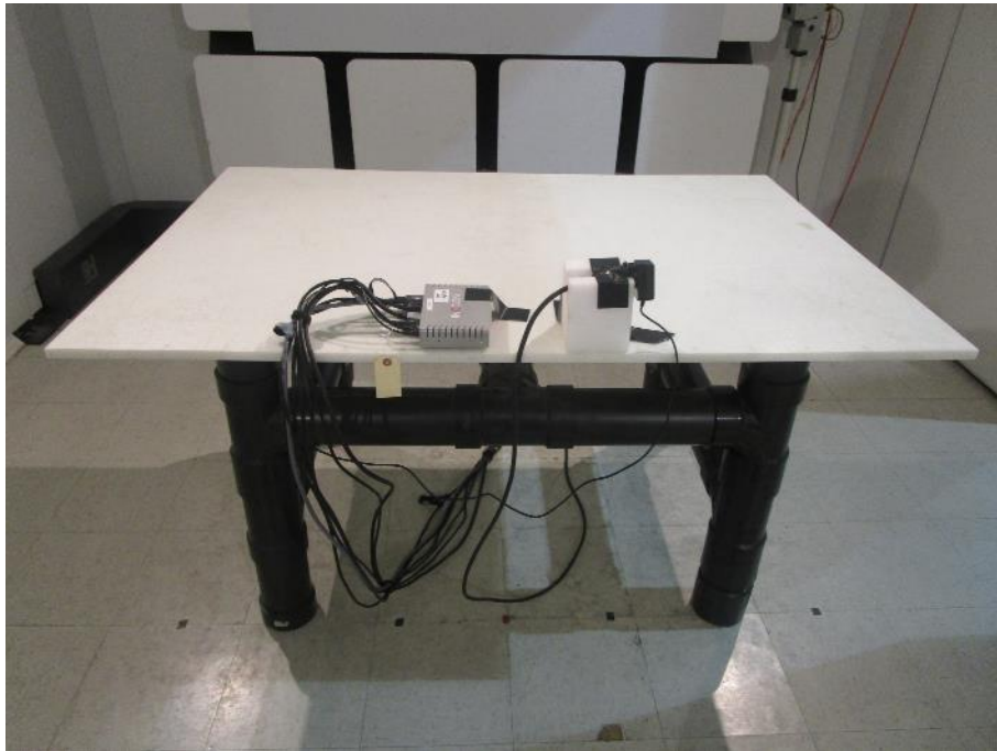
Photo 26: Radiated EM Field – Test setup – Left
