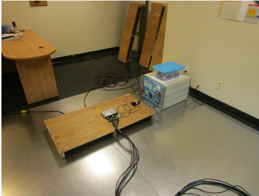
Photo 31: 1.2/50 \mu s Surge – Test Setup
