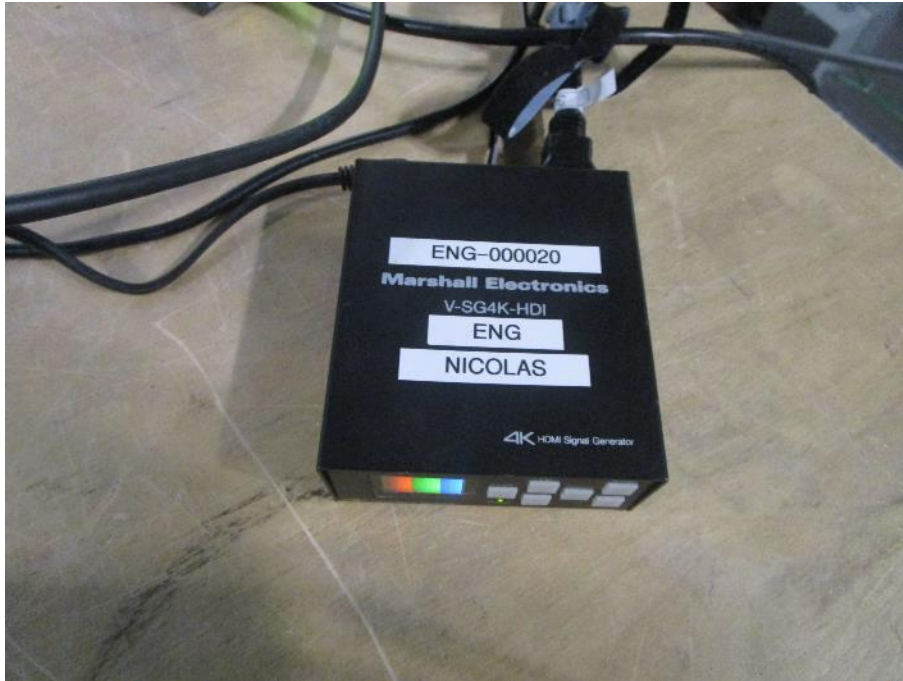
Photo 7: Support Equipment – Video pattern generator
