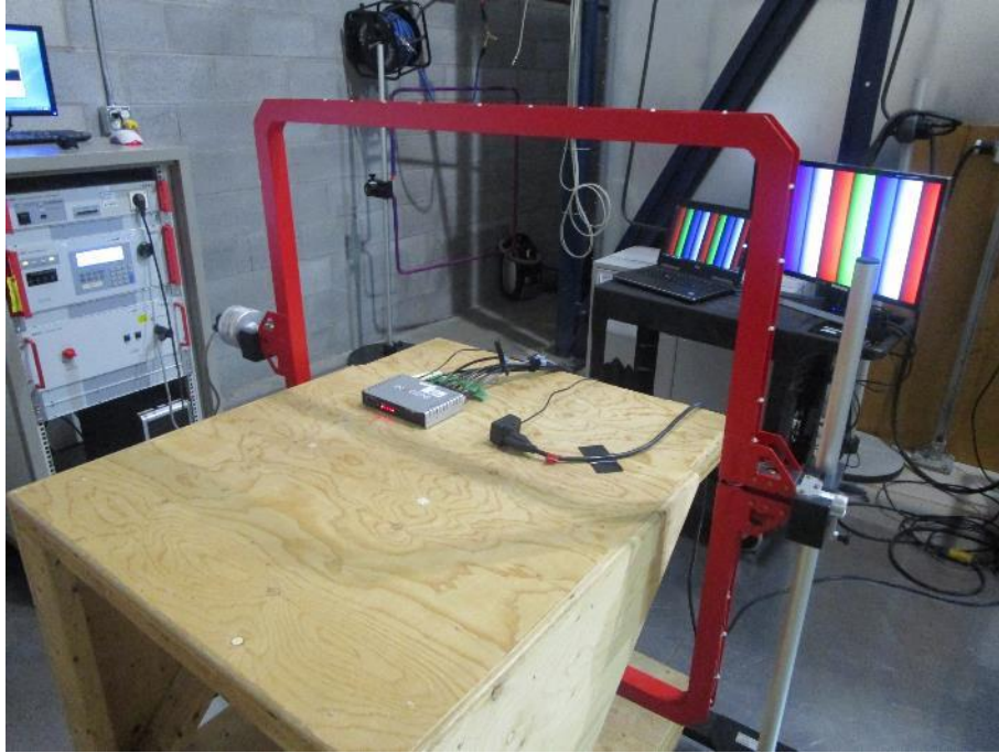
Photo 37: Magnetic Field – Test Setup – Position #1
