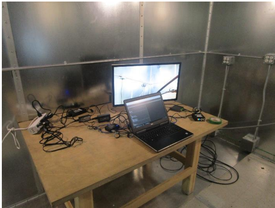
Photo 17: Radiated Emissions – Support Equipment
