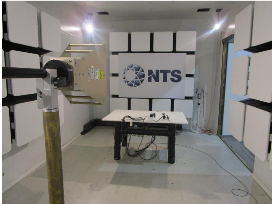
Photo 27: Radiated EM Field – Test setup – >3GHz
