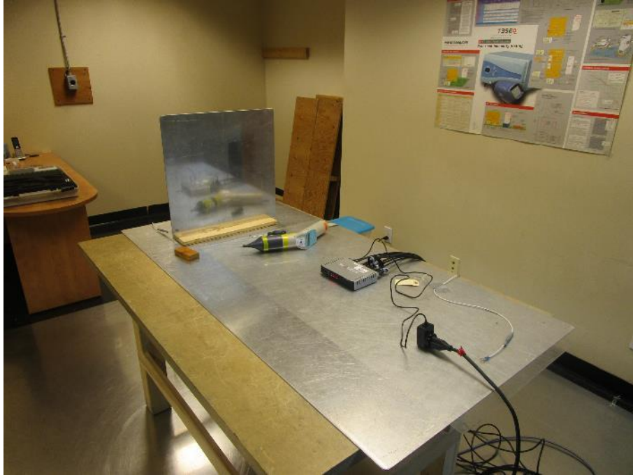
Photo 19: ESD – Test Setup
