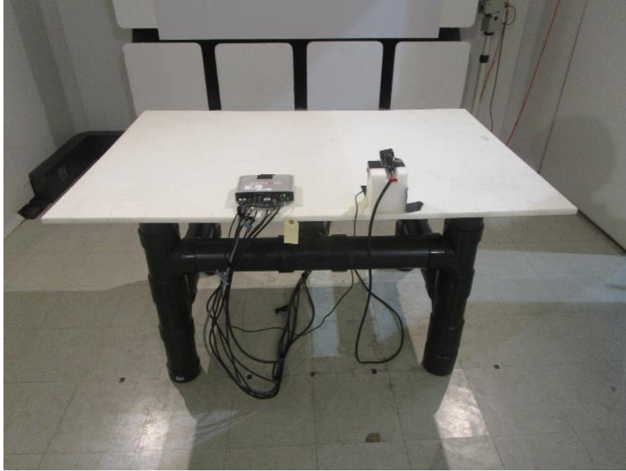
Photo 25: Radiated EM Field – Test setup – Rear
