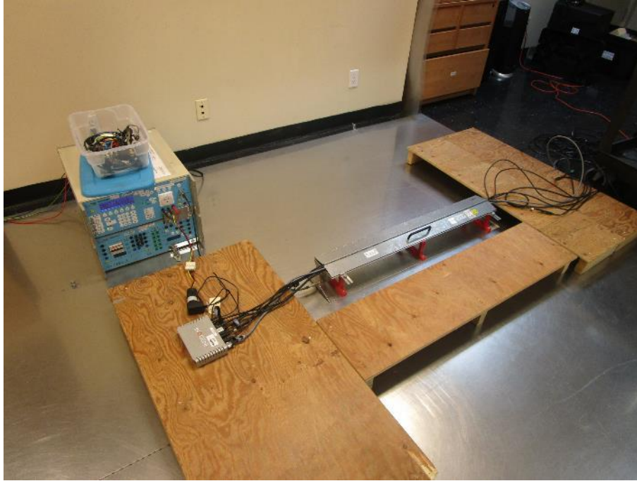
Photo 30: EFT – Test Setup – Capacitive Clamp – All cables
