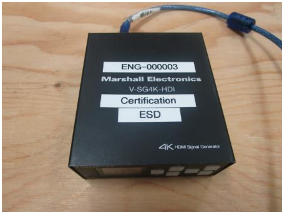
Photo 7: Support Equipment - - HDMI Generator #2
