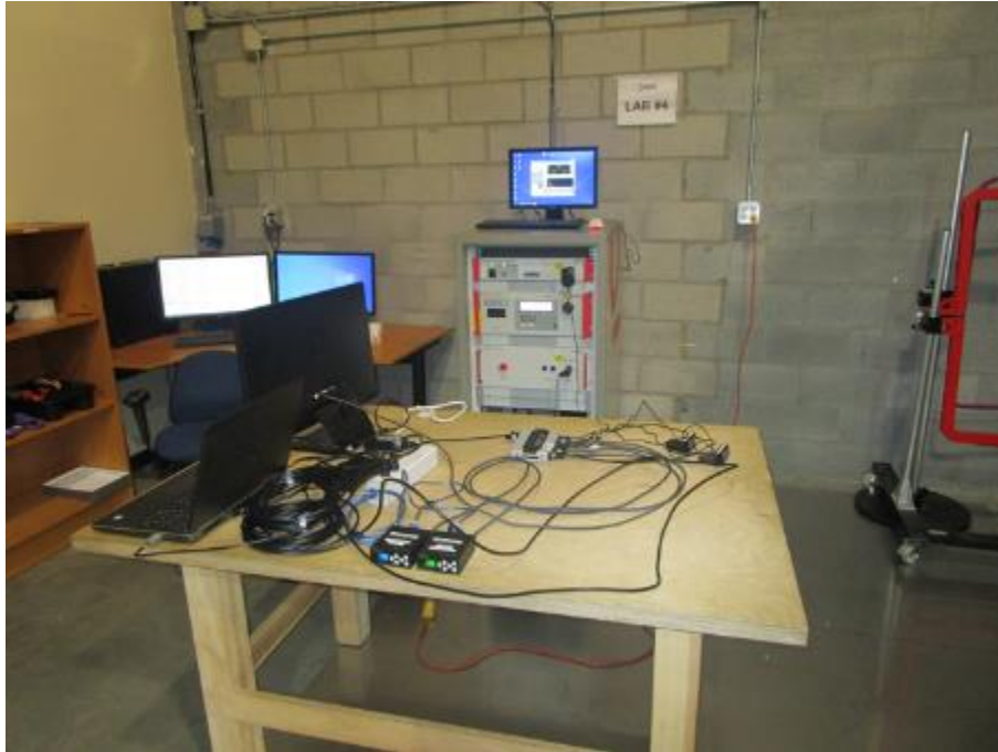
Photo 16: Harmonic Current Emissions – Test Setup
