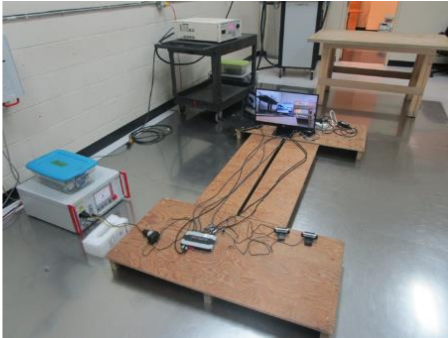
Photo 39: Voltage Variations on AC Input – Test Setup
