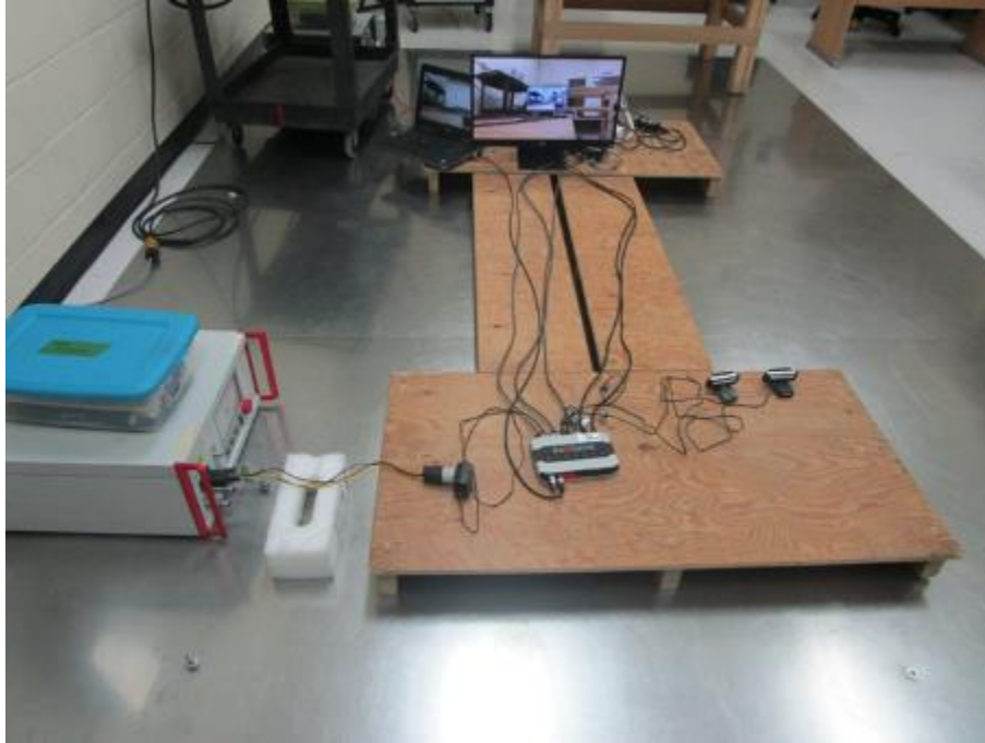
Photo 30: 1.2/50 \mu s Surge – Test Setup – Power Ports
