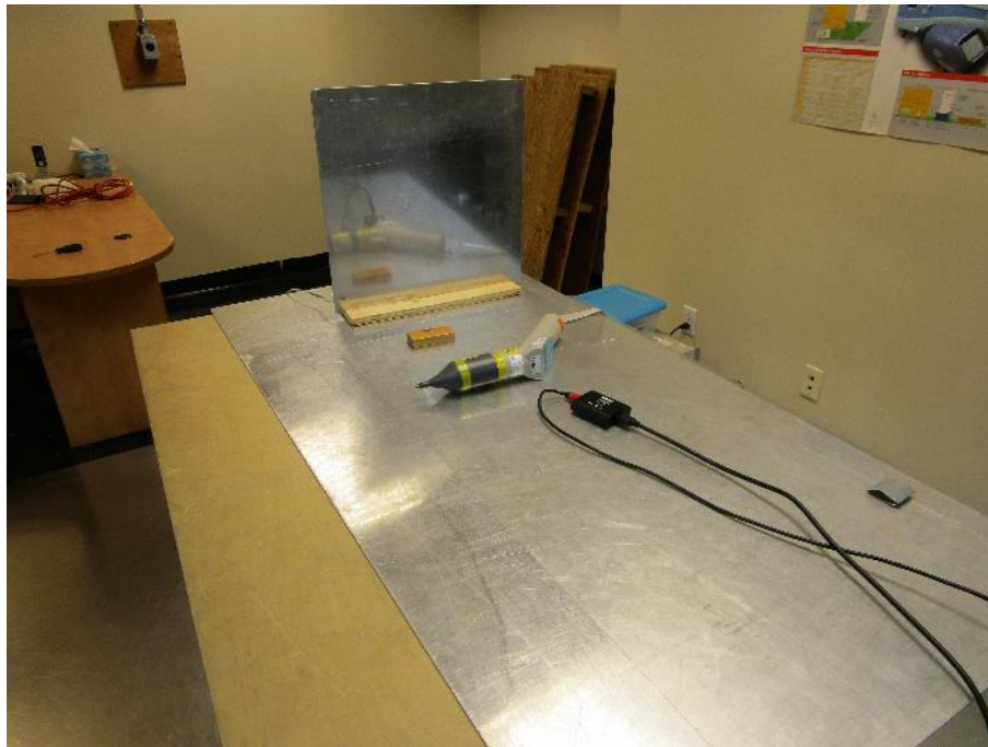
Photo 9: ESD – Test Setup
