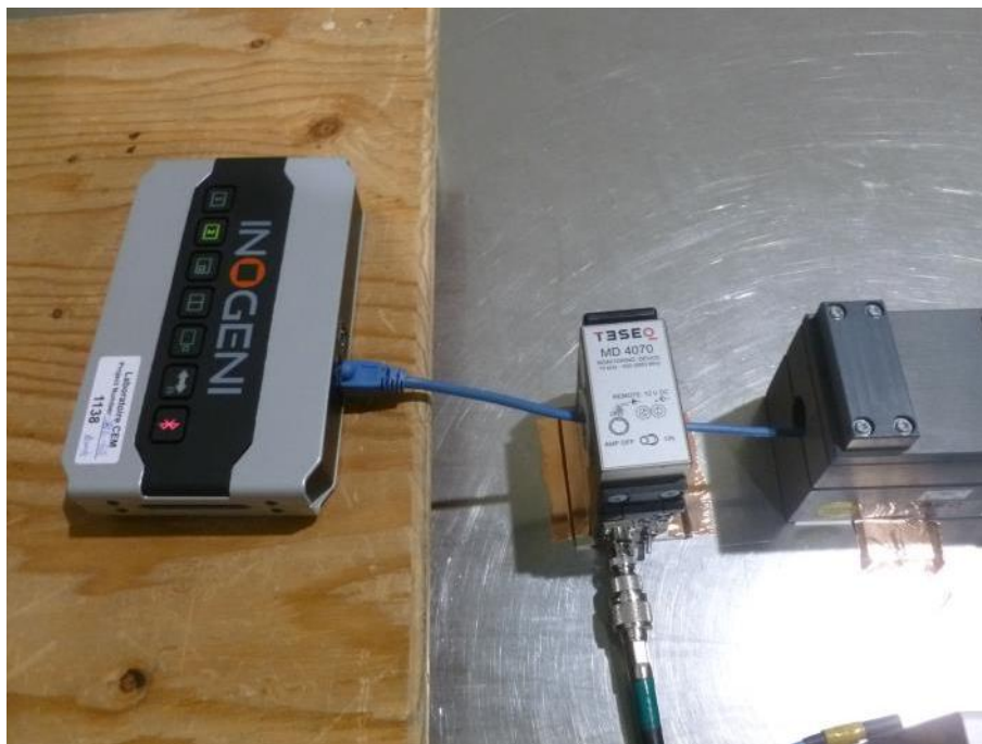
Photo 43 : Conducted Disturbances – Test Setup – EM Clamp – RS-232 (REMOTE)
