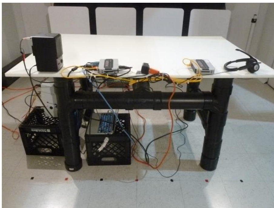
Photo 32 : Radiated EM Field – Test setup – Left
