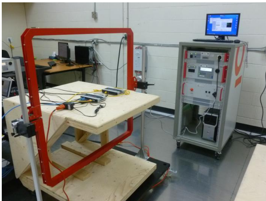
Photo 45 : Magnetic Field – Test Setup – Position #2
