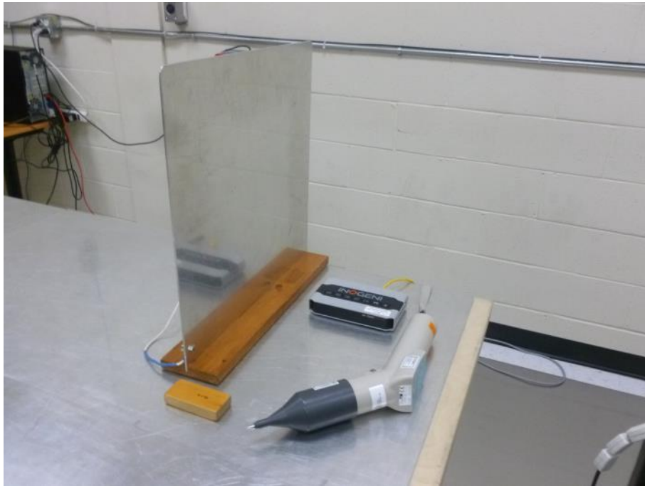
Photo 24 : ESD – Test Setup – REMOTE
