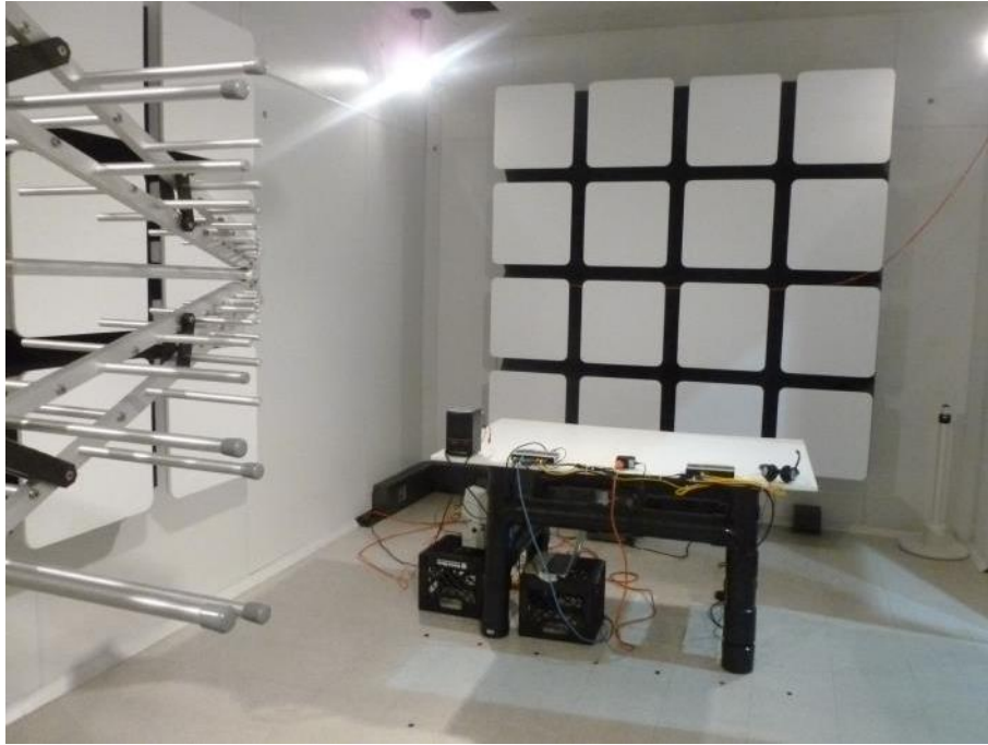
Photo 33 : Radiated EM Field – Test Setup
