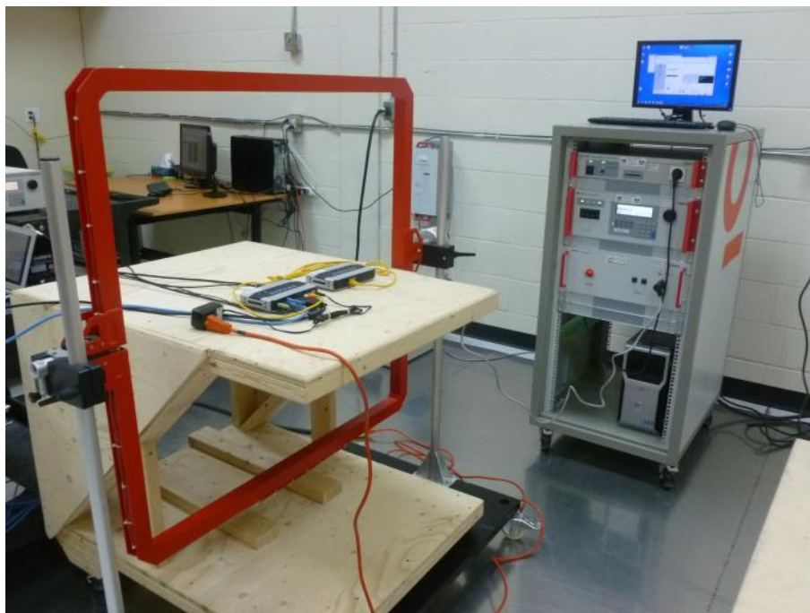
Photo 44 : Magnetic Field – Test Setup – Position #1
