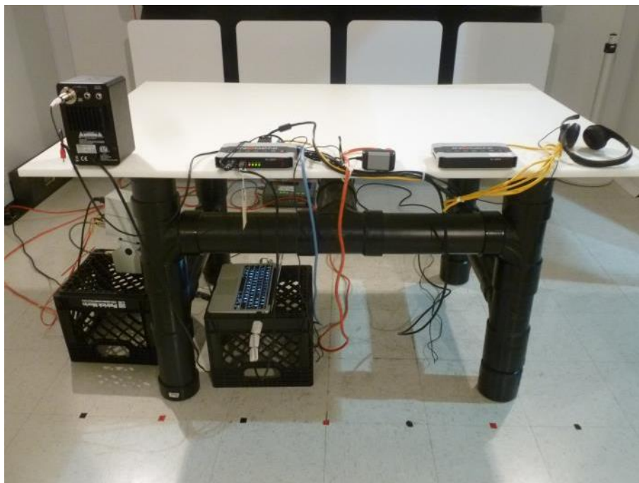
Photo 29 : Radiated EM Field – Test setup – Front
