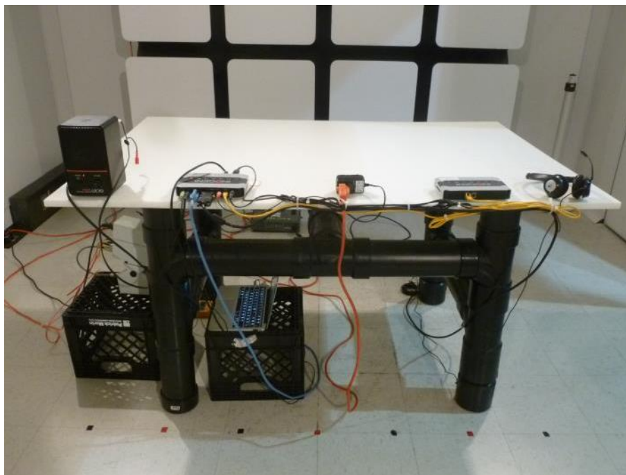
Photo 31 : Radiated EM Field – Test setup – Rear
