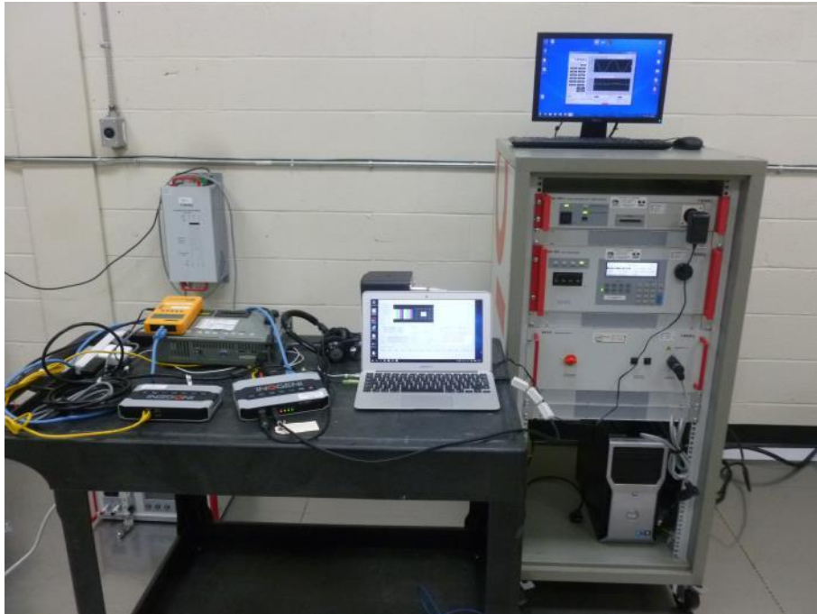
Photo 21 : Voltage Fluctuations and Flicker Measurements– Test Setup
