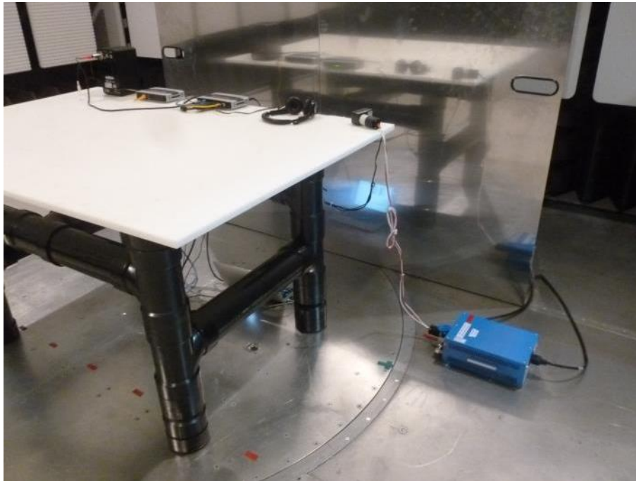
Photo 15 : Conducted Emissions – Test Setup
