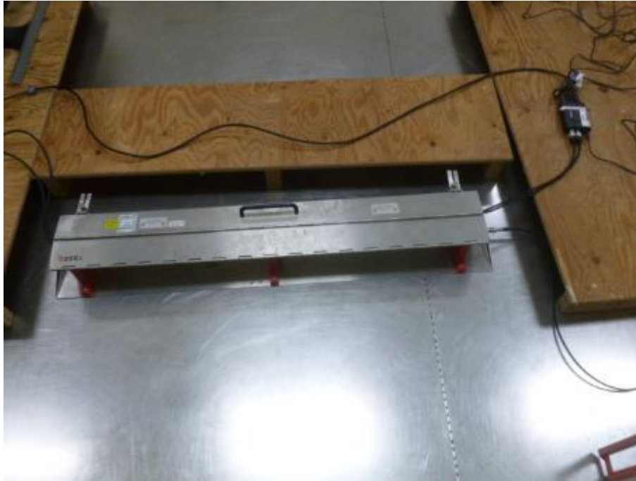
Photo 27: EFT – Test Setup – Capacitive Clamp – PC1 – PC2 (USB)
