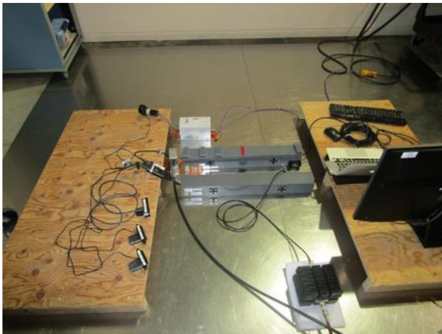
Photo 33: Conducted Disturbances – Test Setup – EM Clamp – Serial
