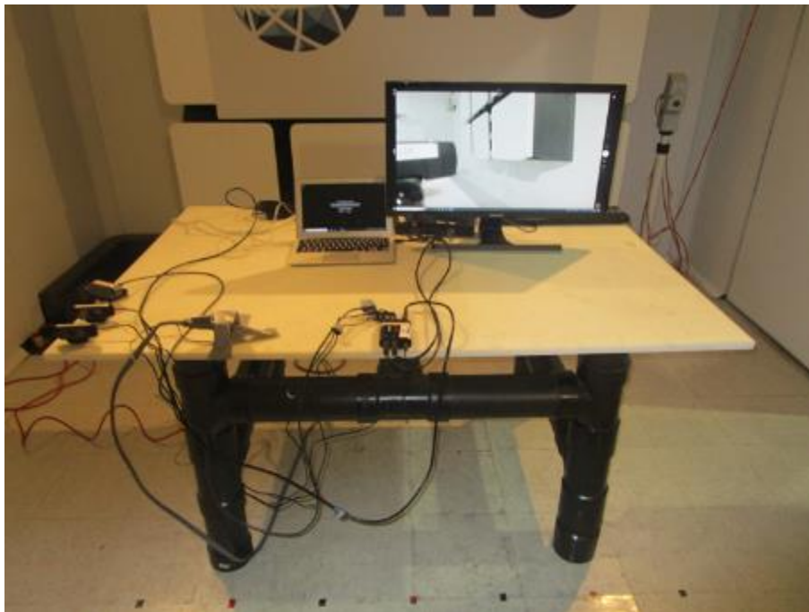
Photo 23: Radiated EM Field – Test setup – Left
