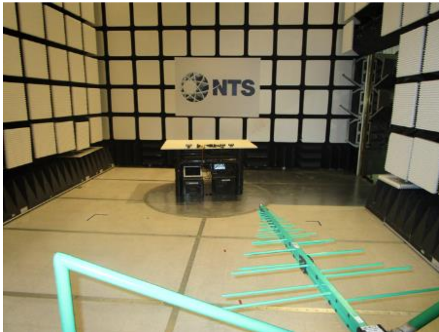
Photo 14: Radiated Emissions – Test Setup 30MHz-1GHz
