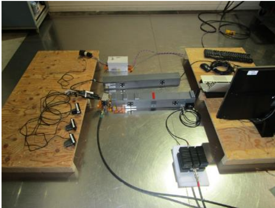
Photo 32: Conducted Disturbances – Test Setup – EM Clamp – PC1 – PC2 (USB)
