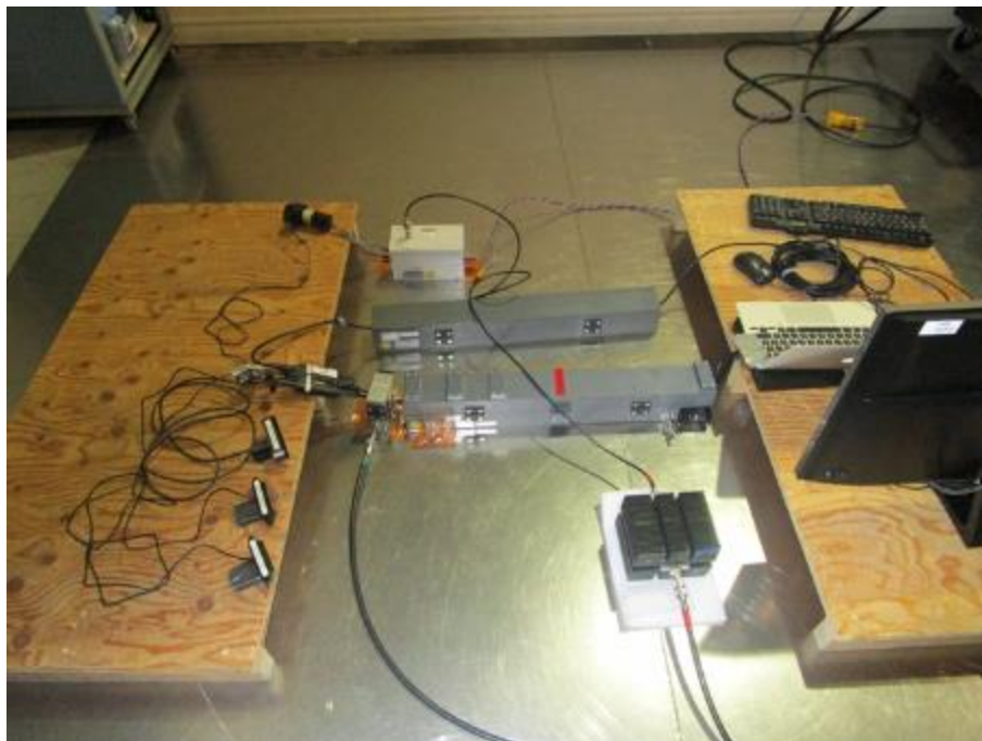
Photo 31: Conducted Disturbances – Test Setup – CDN – Power
