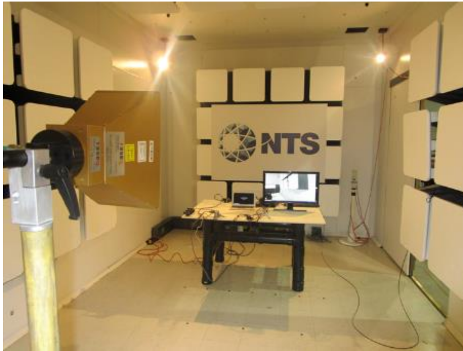
Photo 24: Radiated EM Field – Test setup – >3GHz
