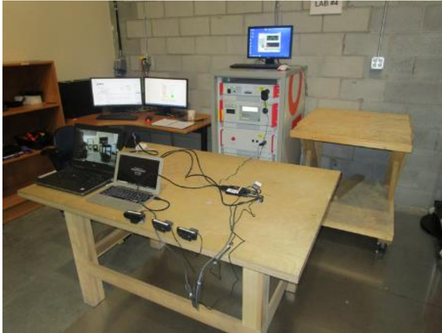
Photo 16: Harmonic Current Emissions – Test Setup
