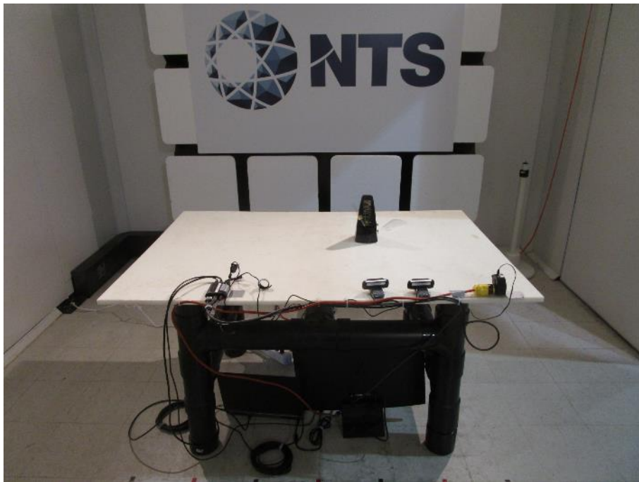
Photo 23: Radiated EM Field – Test setup – Right
