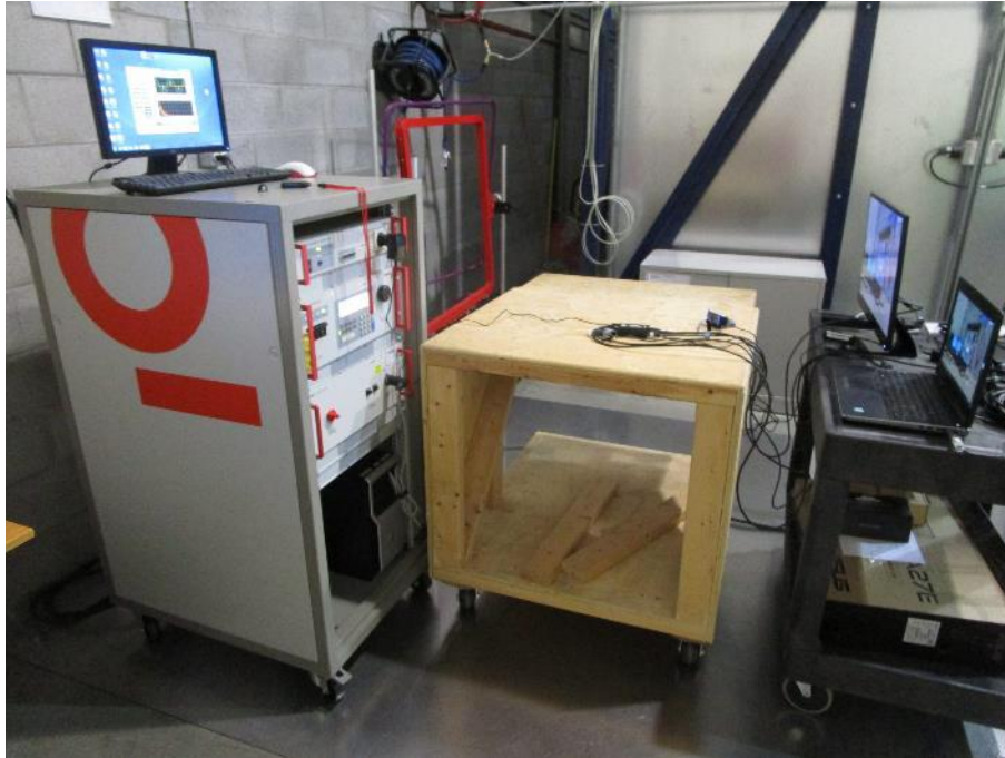
Photo 17: Harmonic Current Emissions – Test Setup
