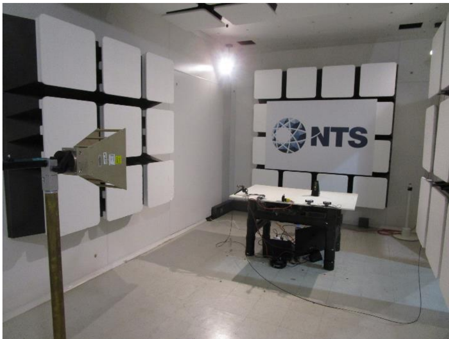
Photo 27: Radiated EM Field – Test setup – >3GHz
