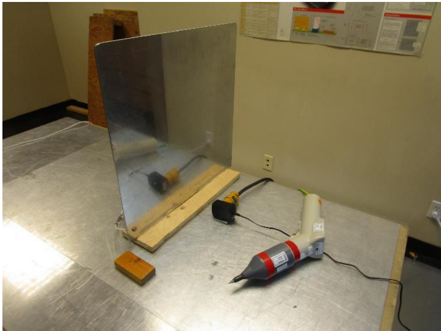
Photo 19: ESD – Test Setup – PSU
