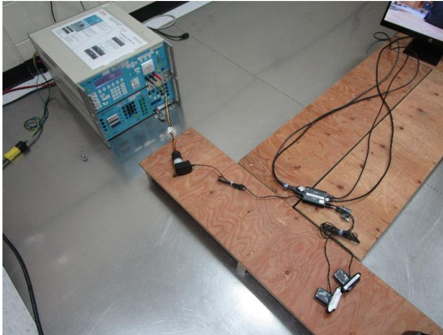
Photo 40: Voltage Variations on AC Input – Test Setup
