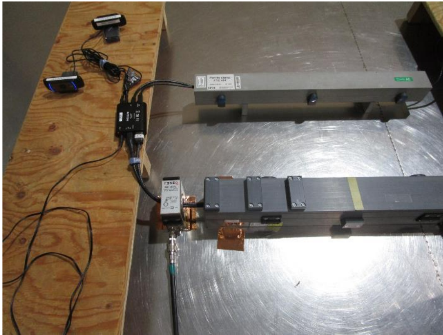
Photo 35: Conducted Disturbances – Test Setup – EM Clamp – Serial & HDMI
