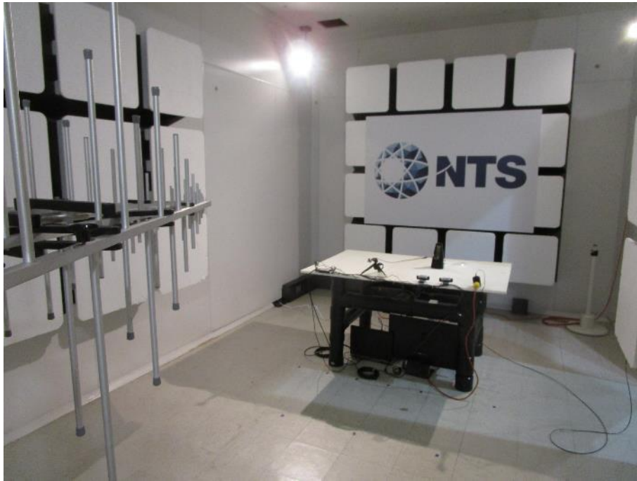
Photo 26: Radiated EM Field – Test setup – <3GHz
