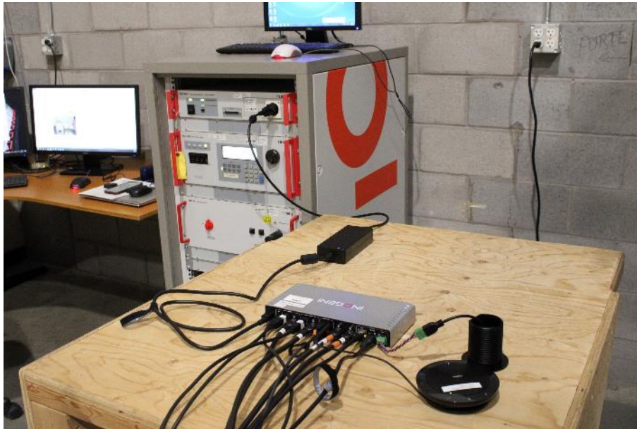
Photo 20: Harmonic Current Emissions – Test Setup
