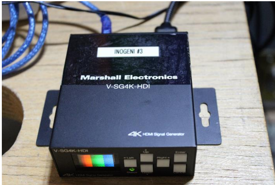
Photo 10: Support Equipment – Video pattern generator
