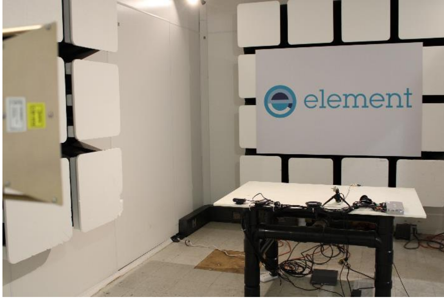
Photo 29: Radiated EM Field – Test setup – >3GHz
