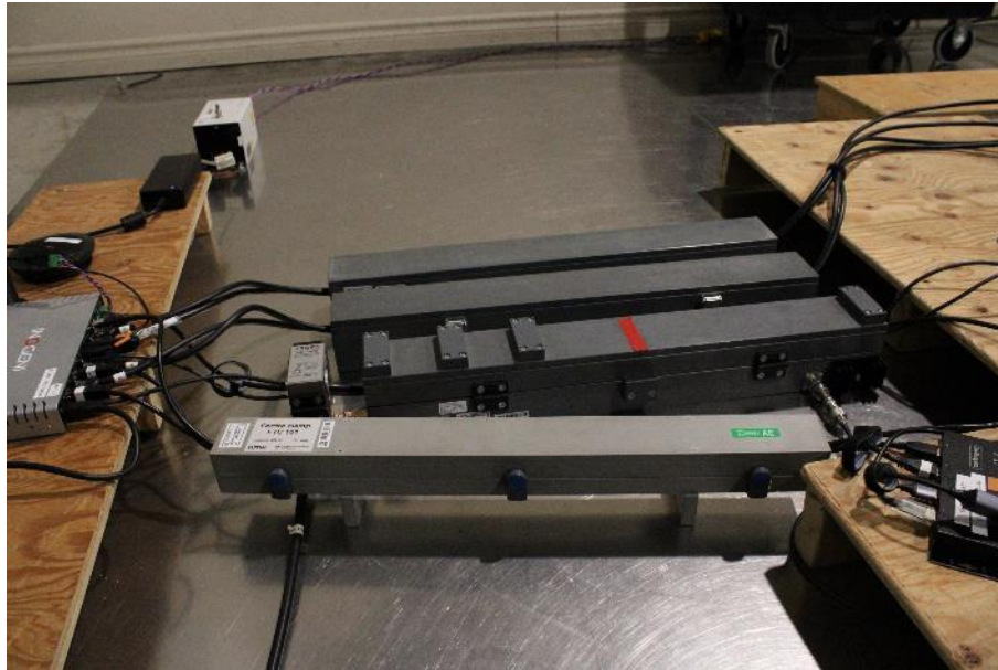
Photo 38: Conducted Disturbances – Test Setup – EM Clamp – RS-232_USB_Ethernet
