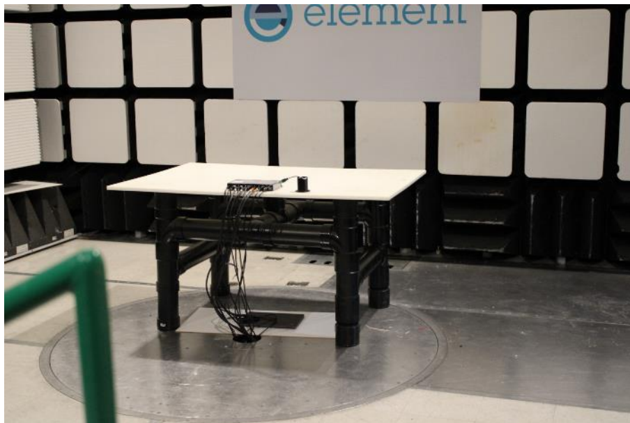
Photo 17: Radiated Emissions – Test Setup 30MHz-1GHz
