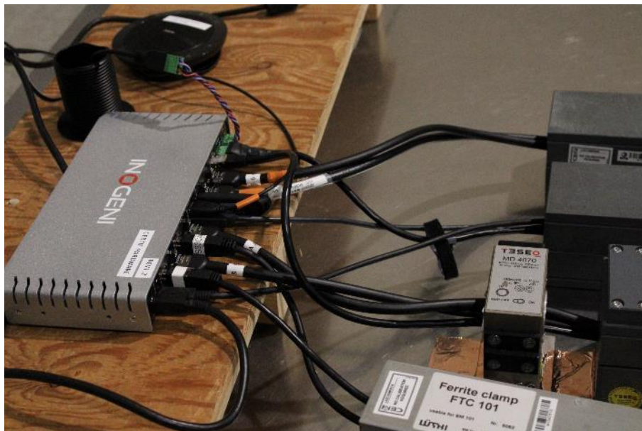
Photo 39: Conducted Disturbances – Test Setup – EM Clamp – HDMI Host
