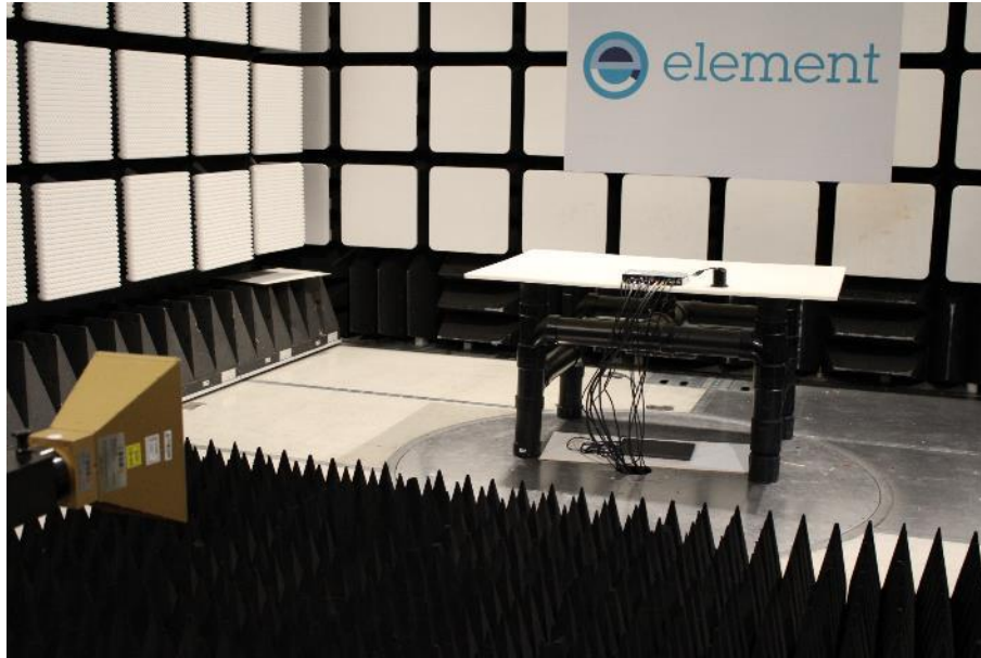
Photo 18: Radiated Emissions – Test Setup 1GHz-2GHz
