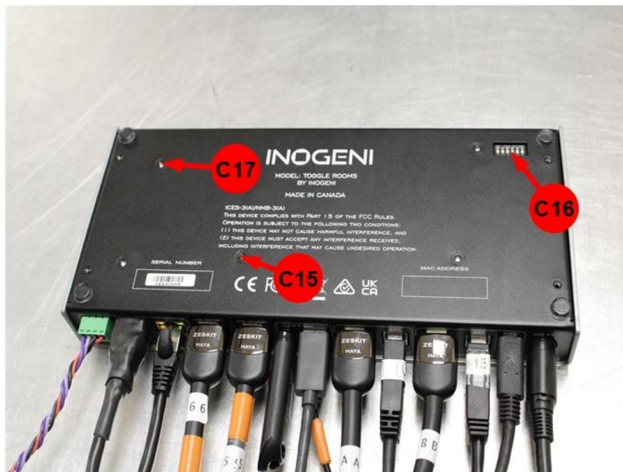
Photo 24: ESD – Location of Discharge Points #3
