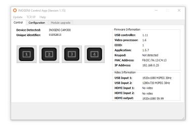
The device has its own application in order to control the Mixer configuration using the USB HID or the LAN interfaces. You can also monitor the firmware versions installed on the device and the status of the USB and HDMI inputs. You can update your device to the latest firmware using the Update menu. The C++ source code of this application is available on demand. Visit the Software Update page under the INOGENI CAM section for more details.
