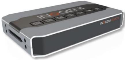
The INOGENI Remote needs to be connected to the terminal block port in order to operate. Apply wiring accordingly. This remote is sending serial commands to the SHARE2U device. Make sure to set the **DIP SW6** below the SHARE2U to ON in order to apply power to the remote before going further. See “DIP SWITCHES” section of this document for more details. Check the user manual of the INOGENI REMOTE for more details.
