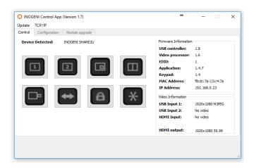
The device has its own application in order to control the Mixer configuration using the USB Human Input Device (HID) or the LAN interfaces.
