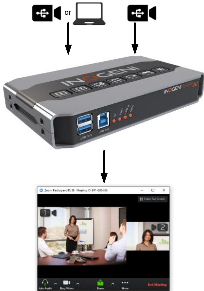
Figure 4: SHARE2U common setup with 2 cameras.
