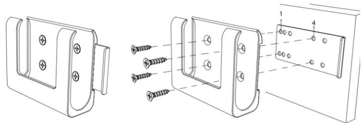
**Screw into holes 2 and directly into the surface**
