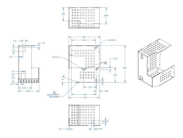
Figure 2: DEVICE module dimensions
