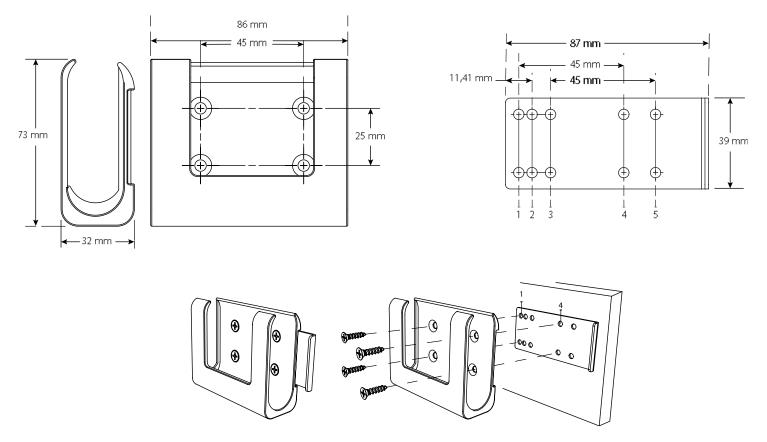
Figure 3: Bracket dimensions for PC host module
