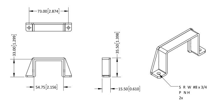
Figure 4: Power supply bracket dimensions
