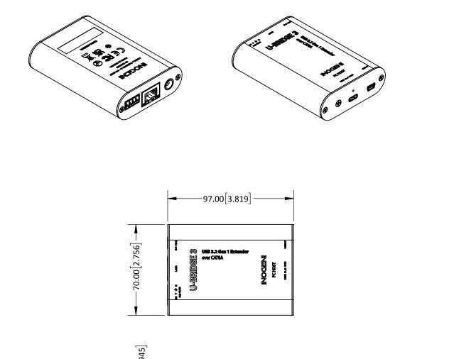
Figure 1: PC HOST module dimensions
