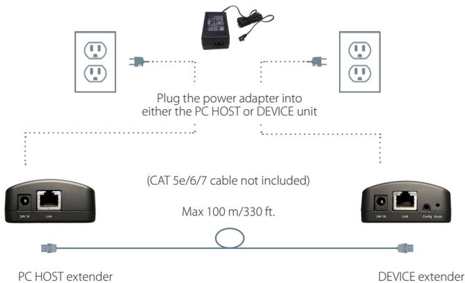
Note: Flexible power is different from Power over Ethernet (PoE). Ensure that the CAT 5e/6/7 cable is only connected between the PC HOST and DEVICE extenders.
