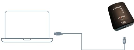
**4** Attach your USB device to the DEVICE extender.
